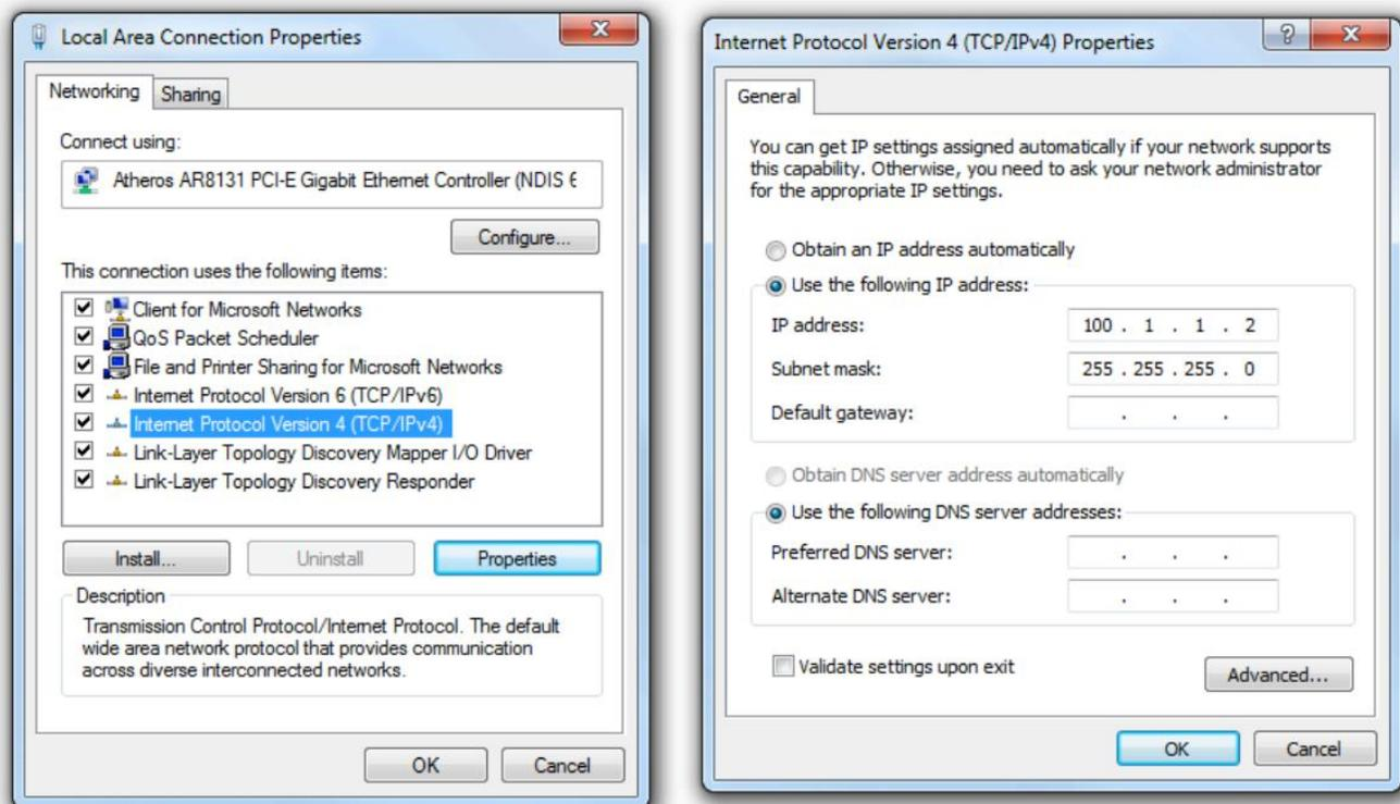
Figure 9-2: Configure IP address on Windows 7
